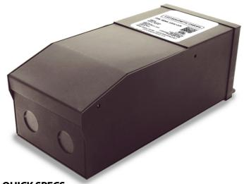
KLUS - MD-300-24 is the most compact LED driver on the market with a magnetic transformer core. It is equipped with two push-to-reset circuit breakers on the input and output, which protect both the load and driver. The driver is encased in a coated metal box that includes 2 knock-outs on the bottom to enable easy installation that complies with electrical code requirements.
